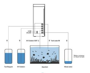
Attach the tubing using the twist lock connectors as shown in the diagram above, matching the coloured hose to the correct coloured port. It is important that any hose connections are properly locked, to avoid air being drawn in. Ensure that the supplied filter is fitted to the end of the green pipe which takes sample water from the sump and is positioned so that the end will always remain submerged but will not draw in debris which may clog the hose and cause false test results.
