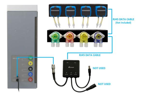
The E1 Connection Box can be used to link one or two D-D P4 or P4PRO dosing pumps to the KH manager, If two pumps are used they can be of the same type or one P4 and one P4PRO.
