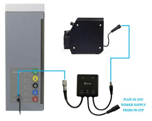
Connect the 'Click Lock' connector to the back of the KH Manager by aligning the locating ribs and pushing into place. **Excessive force must not be used when making the connection as it may damage the terminals.** To remove the connector at any time, pull back on the outer metal cover of the connector and it will slide back and release the connection.
